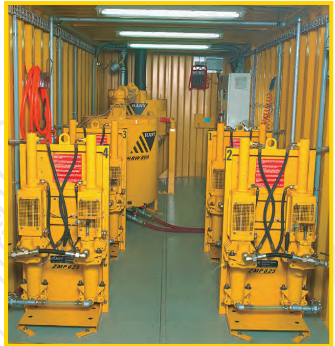
MCI 1400/625 Grout Plant with automated weigh-batching.
