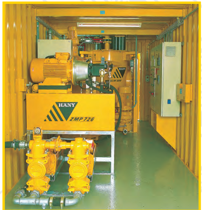
MCI 2000/726 Mixing and grouting plant for soil-mixing.
