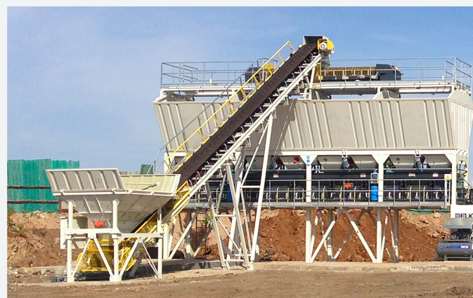
Shuttle Type Automated Aggregate Feeding System
