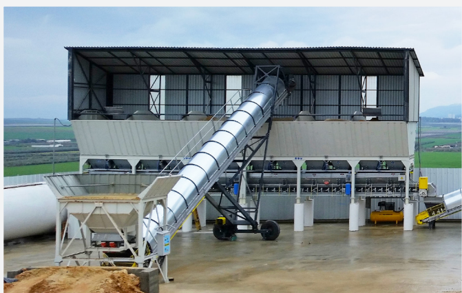
Radial Type Automated Aggregate Feeding System
